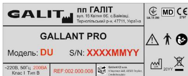
Fig.1.1.1 Identification name plate for dental units with upper delivery of the instruments
