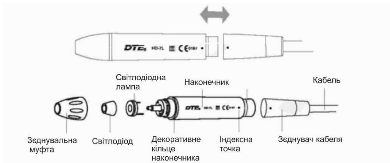
Figure 5.2.4.7 – structure of the LED scaler
